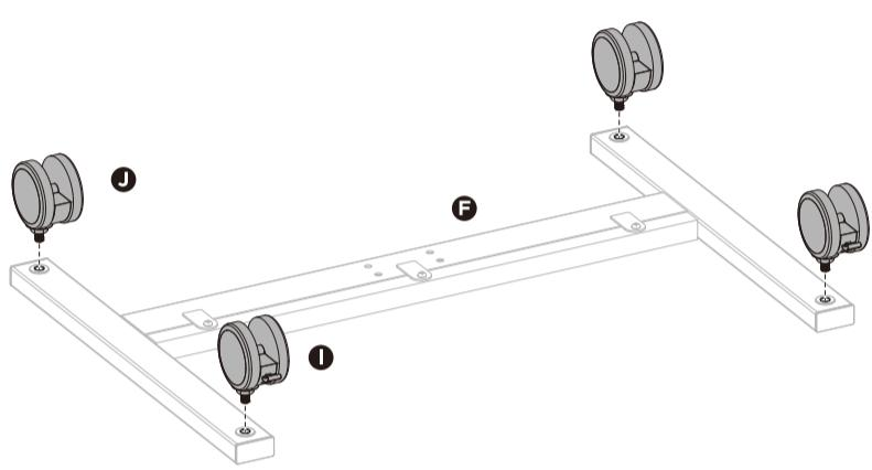
**Note:** The longer side uses casters with brake **I**, the shorter side uses normal casters **J**.
