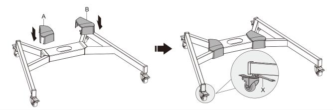
NOTE: Lock the brakes on the casters to avoid any sudden movements during installation.
